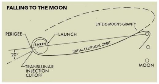
Going to the moon requires getting into a high elliptical orbit (dashed line in diagram). A speed of 35,505 feet/s (10,822 m/s) must be achieved when the booster engine is shut down. If nothing else were done, Apollo 11 would pass behind the moon and then fall back to Earth (a "free return" trajectory). Instead, firing a rocket engine firings puts Apollo into orbit around the moon.
